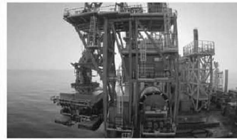
Launch and Recovery System (LARS), Photo: TMC/Alseas
